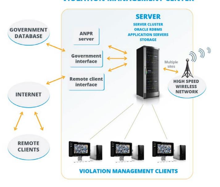
image container. It maintains communication with the Automatic Number Plate Recognition Server, the Government database and transmit violation packages to the violation management clients.
