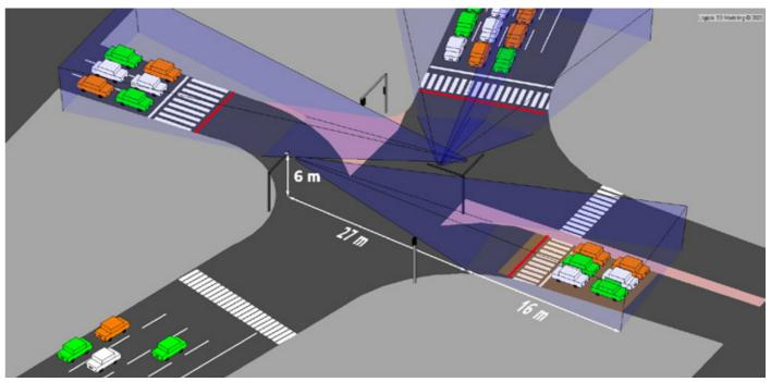
After calculating the required resolution for the desired surveillance task, we create the accurate 3D model of each site with exact camera installation spots and generated camera views.
